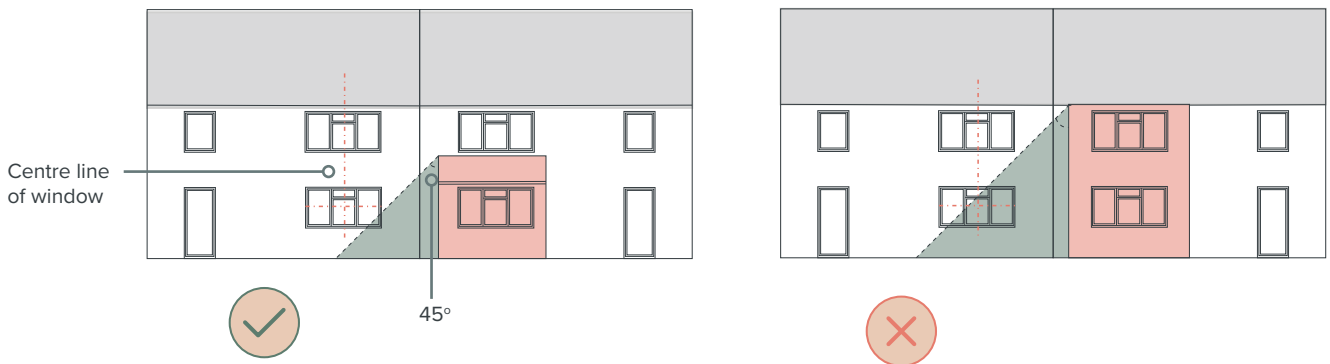
Acceptable and unacceptable massing using a 45° line to the neighbouring window: plans and rear elevations
