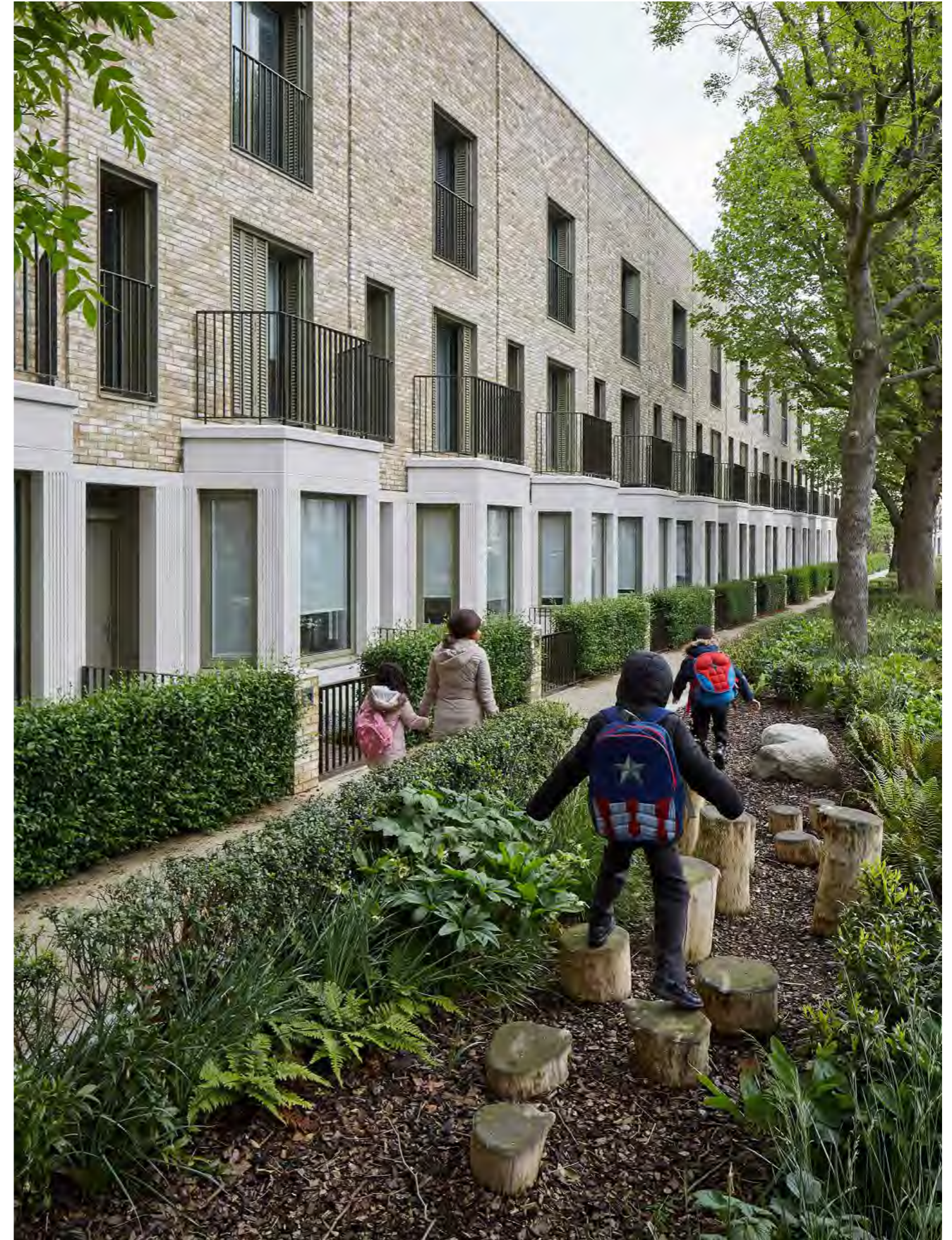
Fig 100 Planting edge to front gardens with inset railings to maximise passive surveillance from ground floor windows
